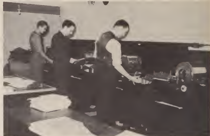
A section of the Duplicating Room in Radio City. Left to right, James Ware, Alfred Patkocy and Edwin Breen are shown operating mimeograph machines each of which turns out 115 mimeographed sheets a minute. Each stencil from which the copies are made is good for 15,000 copies.
