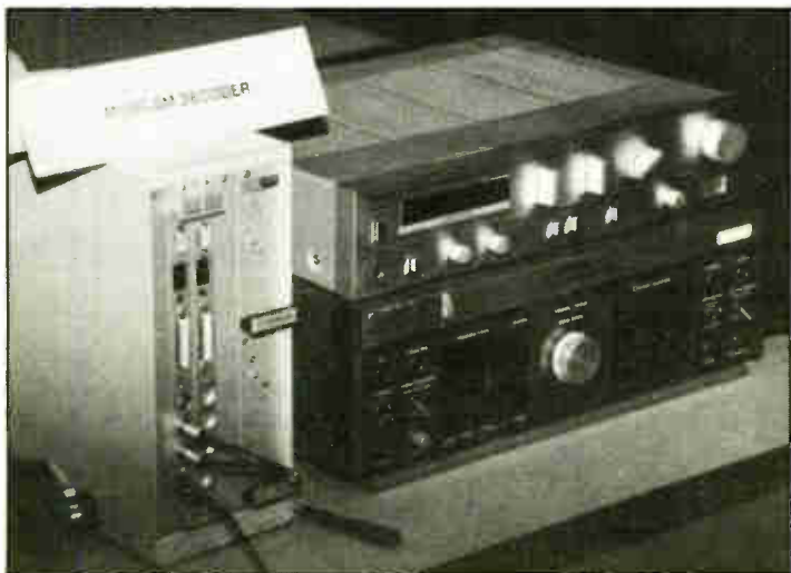
The MUSICAM decoding process reconstructs the audio signal with a bandwidth up to 24 kHz, by using a filter network.
