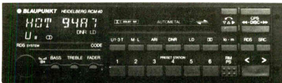
Blaupunkt exhibited an RDS receiver that can display a station's call letters.
