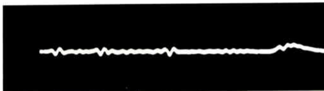
The sine wave shapes echoes seen from left to right represent hard line bullets. The "hump" located to the right of the picture illustrates a faulty bullet.
