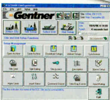
This setup screen allows all parameters to be setup for each site and each I/O unit.
