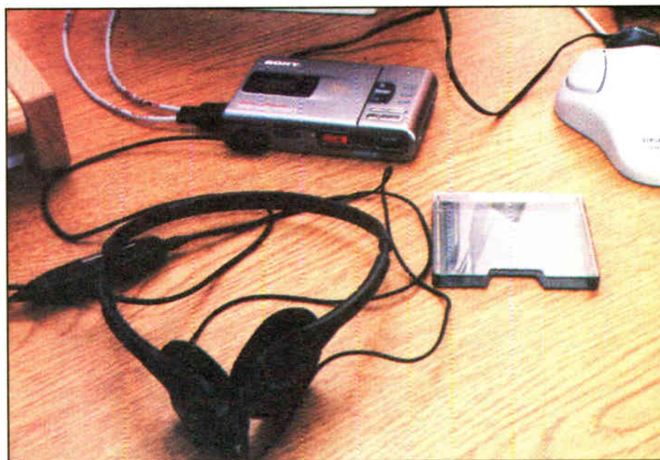
Figure 2: Use a Sony MiniDisc deck to record calls, traffic feeds and remote broadcast bits inexpensively.
