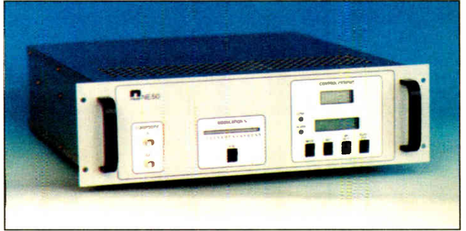
Digital FM exciters like the Nautel NE50 can make a big difference in your sound. They can also be misused.
