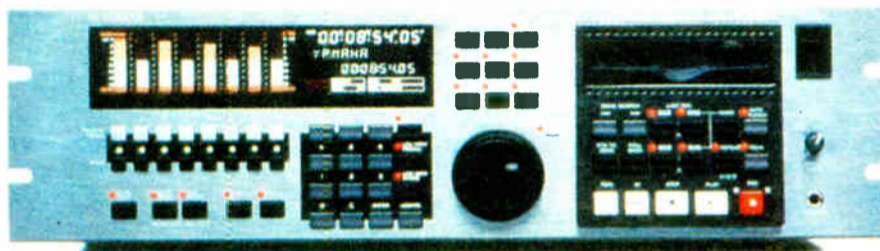
Fig 9: Shown is the Yamaha D24, with eight digital tracks on an MO disk.
