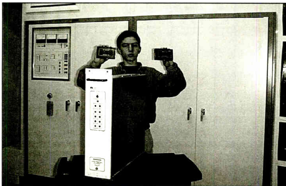
The author's son Lance holds small transistor modules that plug into the XL60 power module.
