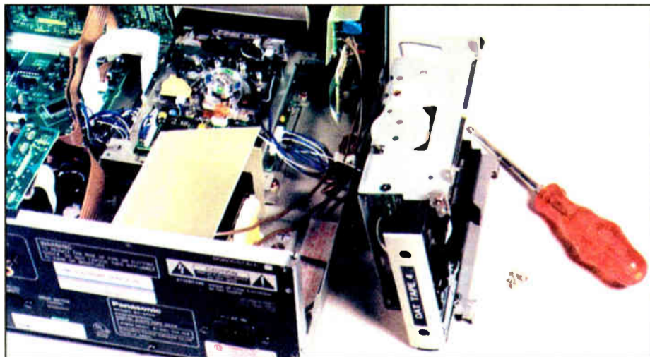
Panasonic: The loading sled is removed and laid aside. Electrical connection is maintained to allow alignment operation of the mechanism.
