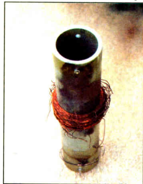
Figure 2: The static drain choke also collapses.
