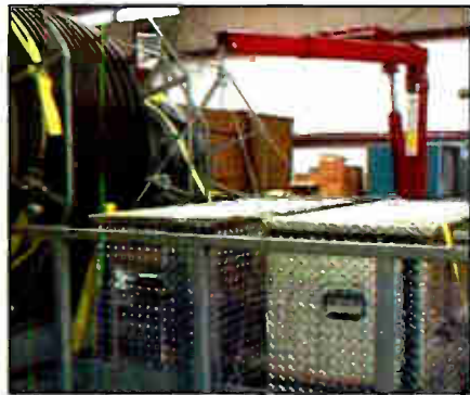
Photo 3: Hand crane lifting custom aluminum cargo boxes
