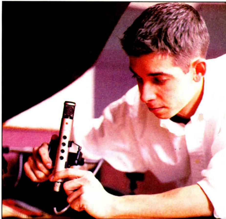
Joe Kloss is shown miking the 6'2" Baldwin conservatory grand piano for a live performance with a Sennheiser MKH800 microphone.
