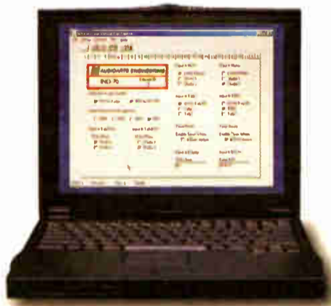
WHEATSTONE'S VDIP™ Virtual Dipswitch Software lets you configure D-70 input channels with a laptop computer. Once configured console runs stand-alone.
