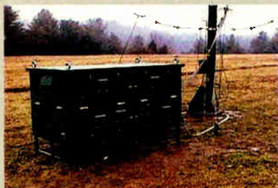
Model STM-AMAB-5K 5 kW All-Band Antenna Tuning Unit And Associated Telescopic Mast
