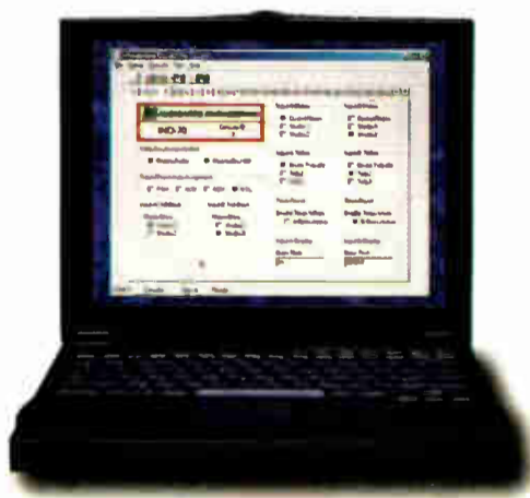
WHEATSTONE'S VDIP™ Virtual Dipswitch Software lets you configure D-70 input channels with a laptop computer. Once configured console runs stand-alone.
