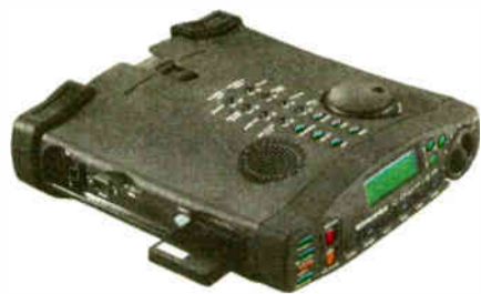
Challenging the traditional analog cassette format are devices like the Sonifex Courier portable recorder, which uses PCMCIA hard disks (PC cards) to store digital audio.
