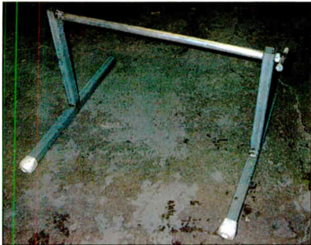
Fig. 1: This collapsible cable reel stand was made at home by Aaron Winski.
