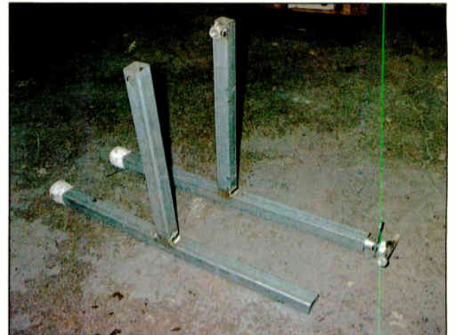
Fig. 3: The sides are made of 1-inch square tubing, welded to form a T.
