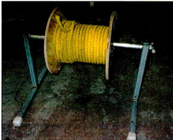
Fig. 2: The stand will hold a reel of 20 inches wide.
