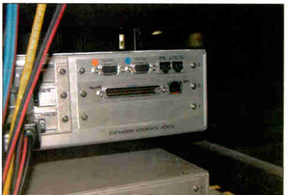
Fig. 2: Remove the multi-pin relay plug on the back of the StarGuide and plug it into the appropriate connector on the relay simulator.
