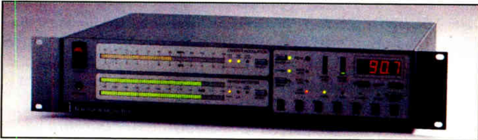
The Model 531 improves upon the earlier 530, with digitally synthesized tuning and a double-conversion design.
