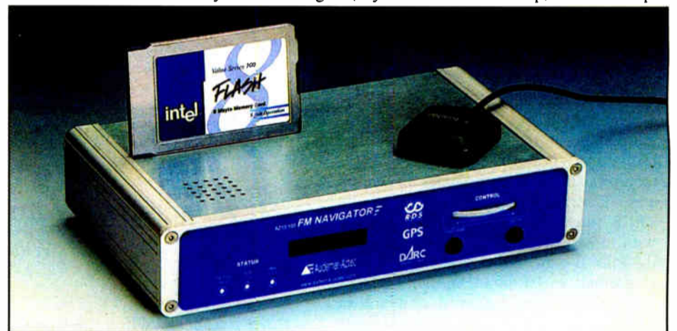
Audemat-Aztec's field strength meter records RF field strength measurements, GPS location and date/time of measurement.
