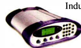
Zephyr Xport is the only POTS codec with aacPlus . It can send 15 kHz mono audio over analog lines.
