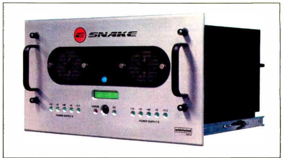
Whirlwind's E-snake uses TCP/IP and the CobraNet protocol to create a link using Cat-5 or IR technology.
