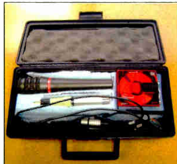
Fig. 3: All of the reporter's tools are accommodated; the foam cutouts guard against any part being left behind.
