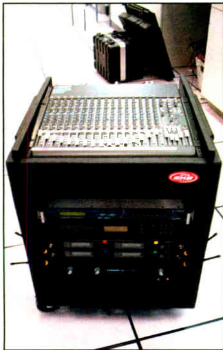
Greater Media engineers in Boston use a self-contained 'Gig-Rig,' a portable rack with mixer, wireless receivers, headsets, POTS codec, ISDN gear and power amp.
