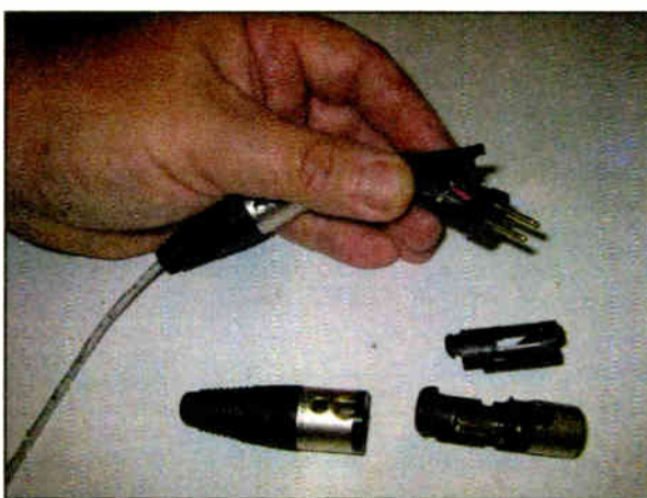
Fig. 2: The Insulation Displacement XLR doesn't need a soldering iron.
