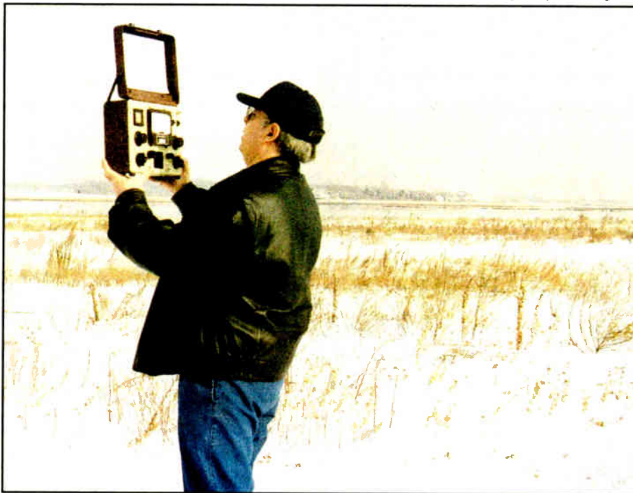
Calibrate before each measurement regardless of how desolate the location. Here, I rotate my meter to identify a peak reading for WFIF(AM) in Milford, Ct.
