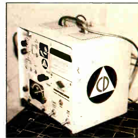
The Civil Defense logo marked not only AM dials but other equipment, like this 'Gooney Box,' a Gonset two-meter ham transceiver. Many of the hams in CD activities were broadcast engineers volunteering as operators on local CD communications networks.
