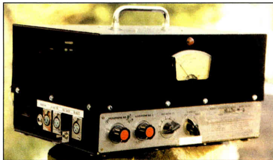
This 160 MHz remote unit, a T/R type designed to work with a receiver for two-way communications, has been refurbished and modified to add an input transformer, selectable mic level switch and headset output.
