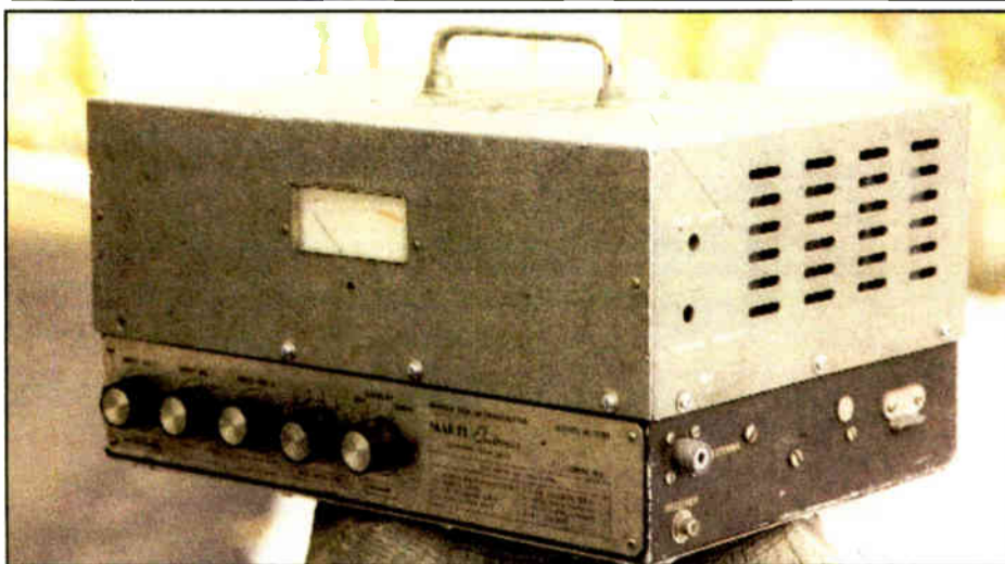
A more recent RPU shows wear and tear. This model had solid-state circuitry all the way to the modulator of the tube transmitter. Output power was 20-30 watts continuous duty.
