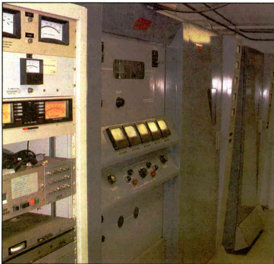
The Gates BC250L transmitter at the radio station from which Arnold purchased it, prior to the move to his house.
