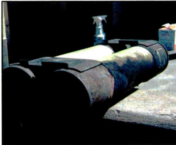
Fig. 2: Two blown fuses thanks to the squirrel's curiosity.
