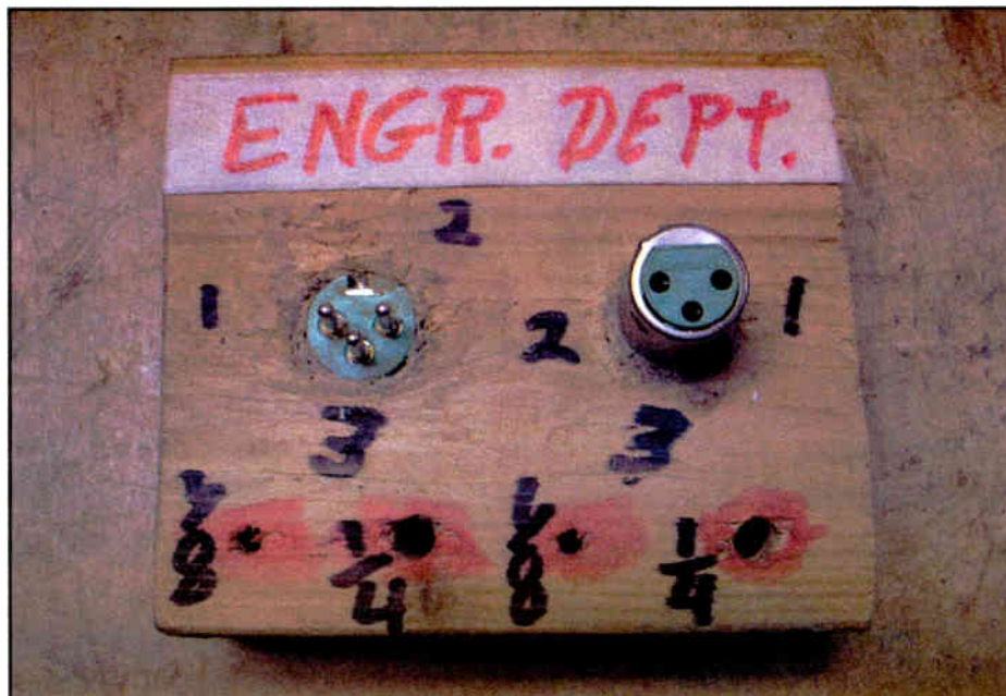
Fig. 3: An economical 'third hand' for soldering.
