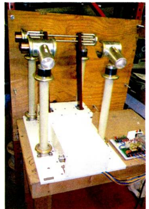
High-Power Linear Actuated Contactor In Prototype
