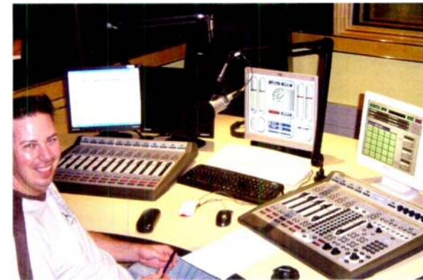
You can easily configure Element to fit your station's unique operational needs. This happy board operator shows off a 24-position, 18-fader split-frame Element at Algoa FM in Port Elizabeth, South Africa.
