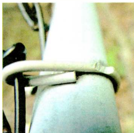
Fig. 2: Squirrels have chewed on aluminum hookup wire.
