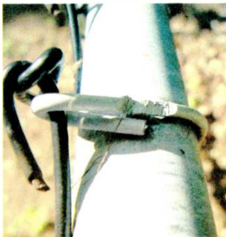
Fig. 1: Teeth marks. Aluminum hookup wire can be damaged by more than sidecutters.
