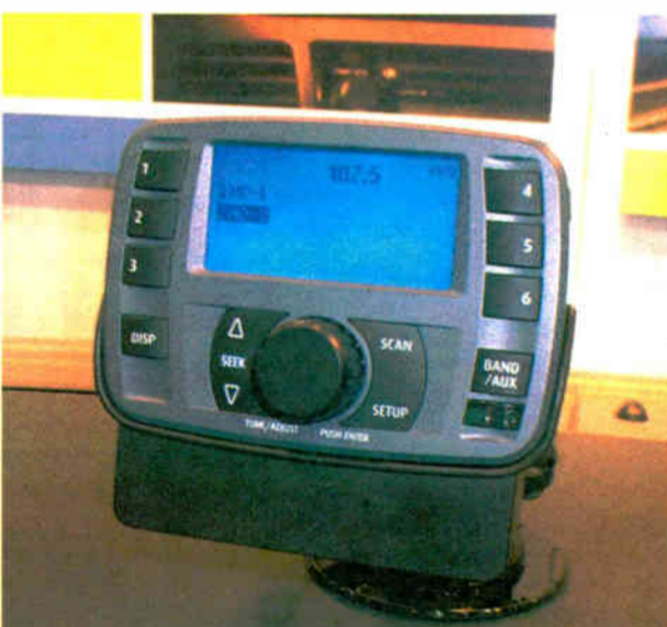
The HD Jump from Visteon can be docked both in the car and at home. The unit is compatible with in-dash head-units from most manufacturers.
