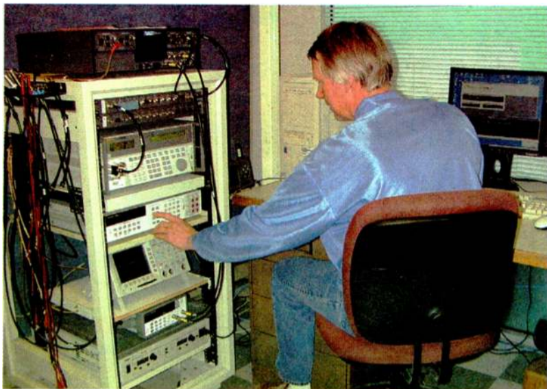
Steve Reeck, manufacturing engineer for Audio Precision, calibrates an AP2712 audio analyzer.
