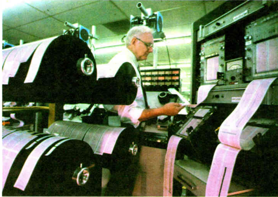
Jim Chestnut performs continuity tests on two-inch analog tape, circa late 1970s. Chestnut worked for Ampex/Quantegy for a number of years, and is now a professional photographer.
