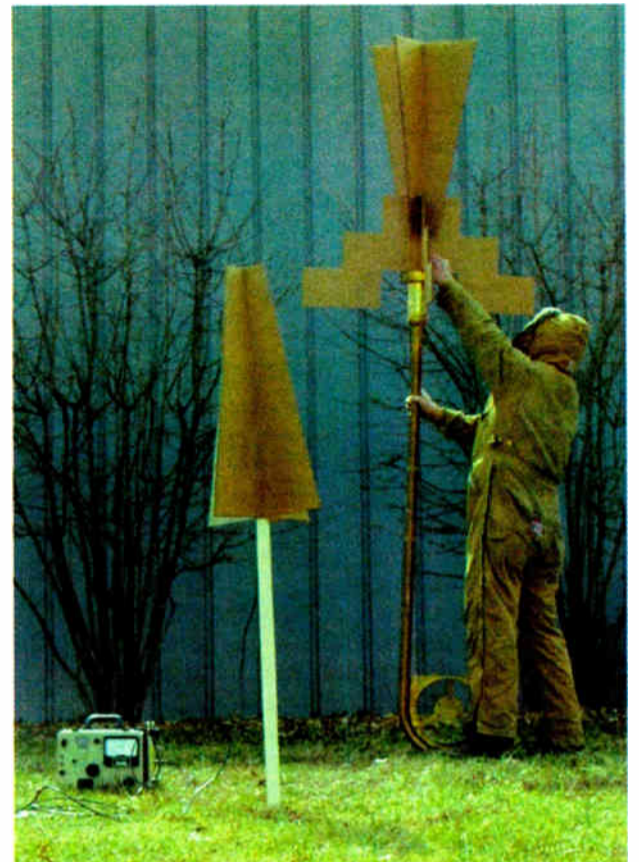
Fig. 1: Milton Silam adjusts the Top Spin Fractal Coefficient prior to making field-strength measurements with a sheet-copper prototype of the TSP antenna. A special receive antenna was attached to an FIM-71 for collecting data.
