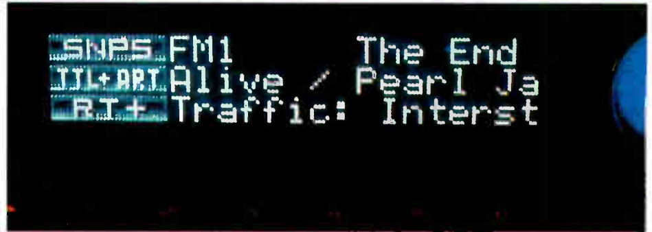
A Kenwood RT+ receiver display with artist, title and traffic text from an analog FM broadcast.
