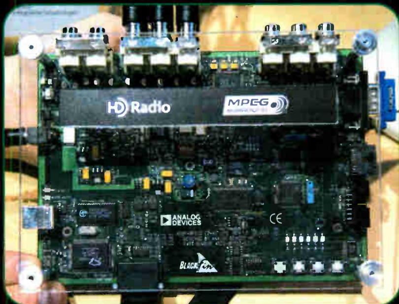
Fraunhofer's new MPEG Surround fixed-point DSP decoder for HD Radio, implemented in a prototype receiver on demo.
