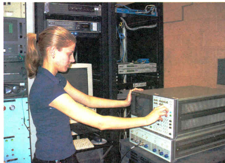
Alexander sets up a spectrum analyzer during an AM IBOC adjustment.
