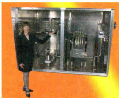
High-Power Antenna Tuning Units
