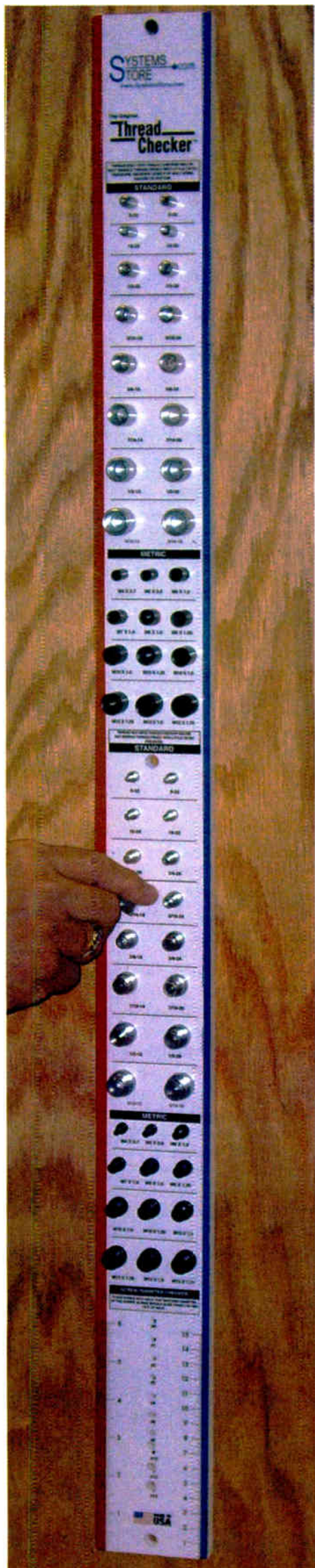
Fig. 3: Quickly determine bolt and nut threads with the Thread Checker.
