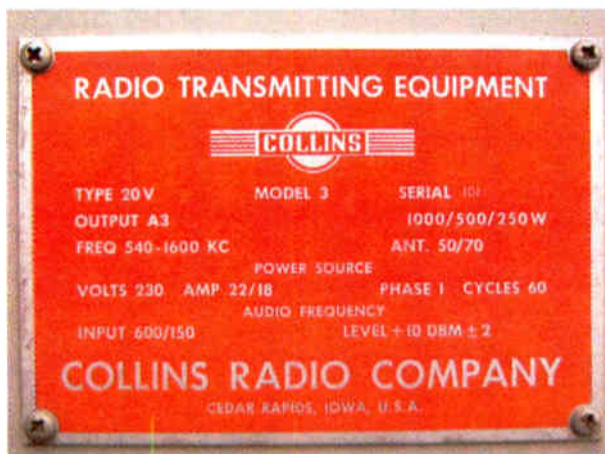
Fig. 1: Manufacturer's plate on Collins 20V-3 serial number 101, owned by Fred Hoffmann, K5OG. It served KSIX(AM), Corpus Christi, Texas for many years and was retired around 2003. Hoffmann said the station offered it to him lest it be sent to a dump.
