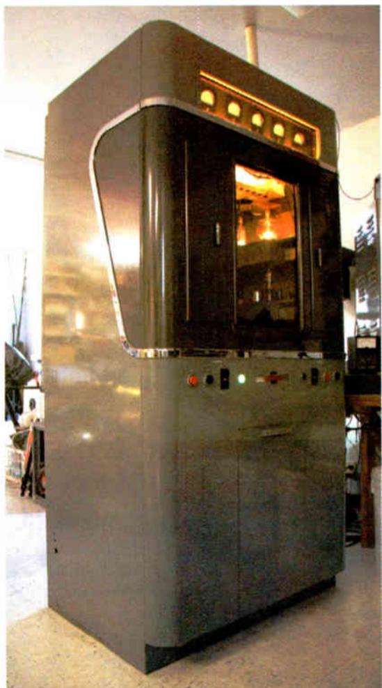
Fig. 2: Chuck Rippel, WA4HHG, provided the photos of his restored Collins 20V-2 seen in Figs. 2-4. It's been retuned and operates crystal-controlled on 1.885 MHz in the 160 meter band. The unit is for sale; contact info is in the photo credit at right.
