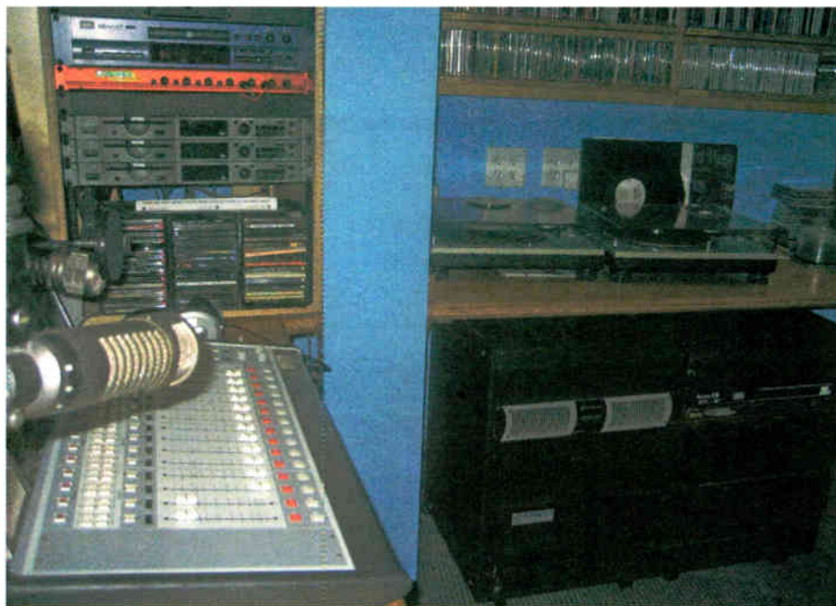
Lasell College Radio uses the AudioTX STL-IP, bottom right, to send audio out and receive audio from the student center's live stage. 'For future use we may even use it with unlicensed band radios to extend our backbone to buildings not on the network,' said Rosenberg.
