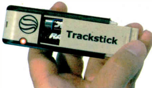
Fig. 1: The Trackstick II provides GPS tracking data and runs for a week on two AAA batteries.
