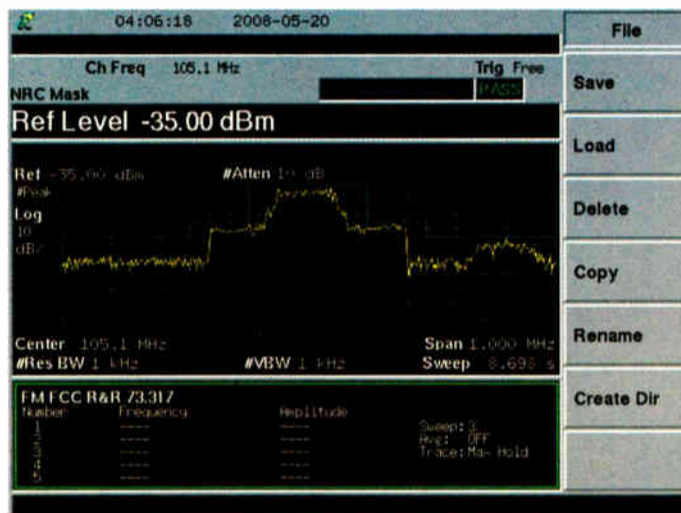
Screen shot showing an FCC occupied bandwidth measurement of an FM station. This station showed a 'pass.'
