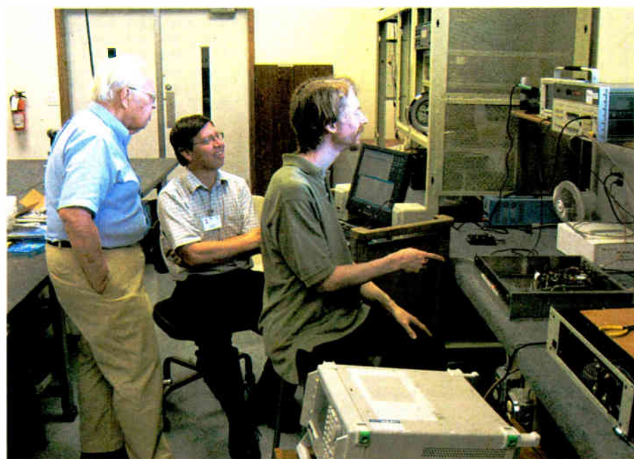
Staff members Herb Jacobson, Charles Jacobson and Peter DeBonte, from left, carry out DRM bench tests with the HCJB low-power shortwave transmitter.
