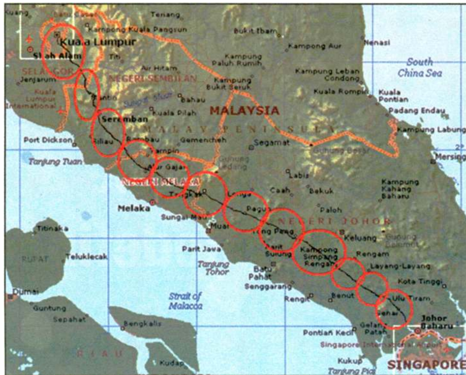
Fig. 4: Several low-powered transmitters broadcasting on the same frequency can provide unbroken service from one end of the highway to the other.
