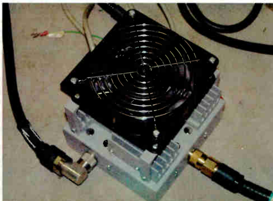
Fig. 2: Keep fans from rotating while you are cleaning with compressed air. A pencil will work (power off, of course).
