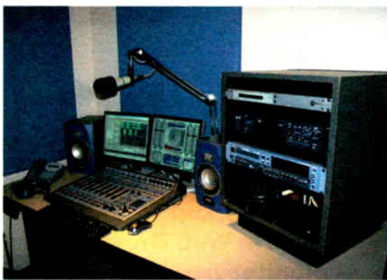
Monitoring in MRN's four audio edit suites is done on Tannoy Reveal 6Ds.
