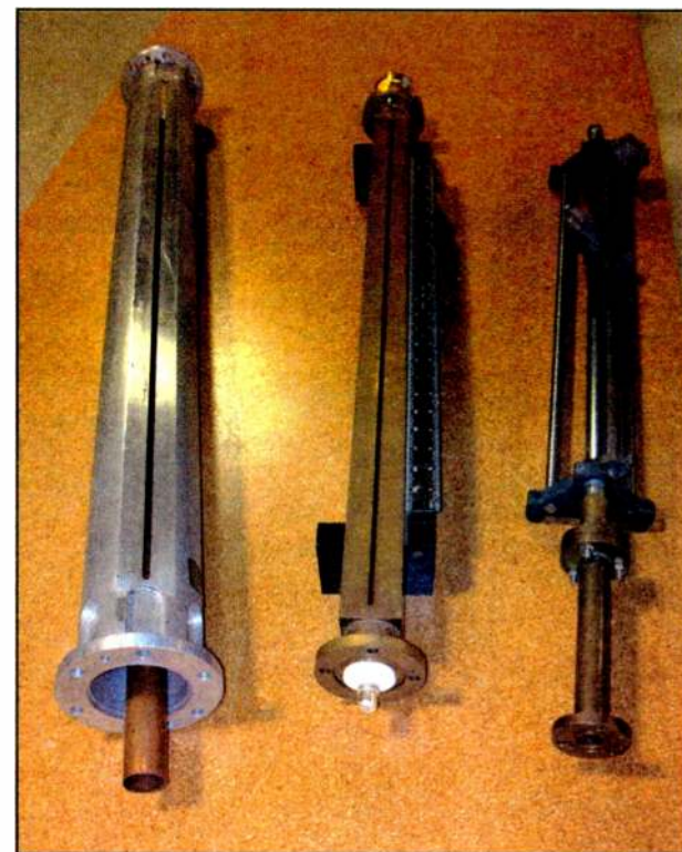
Three slotted lines in 7/8 inch, 1-5/8 inch and 3-1/8 inch rigid line sizes.
