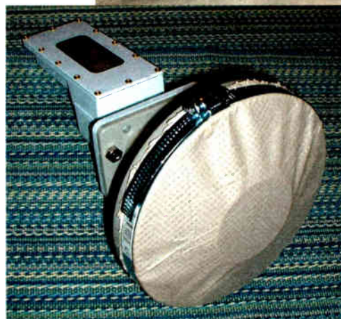
Fig. 4 (above): Hal Schardin's bee-stopper consists of Tyvek house wrap and hose clamps to hold the wrap in place around the satellite feed horn.
