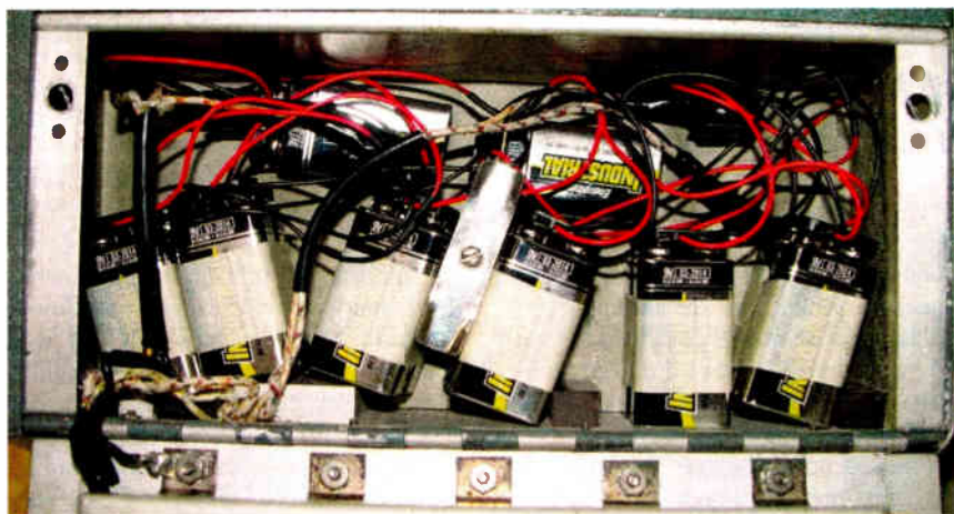
Batteries in an RCA WX-2A Field Intensity Meter. The WX-2C and WX-2D meters don't have the hold-down clamps or fiber spacers.
