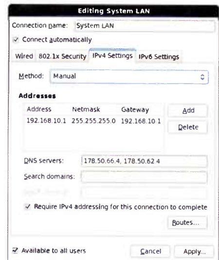
Fig. 2: Setting up the LAN (internal network) side.
