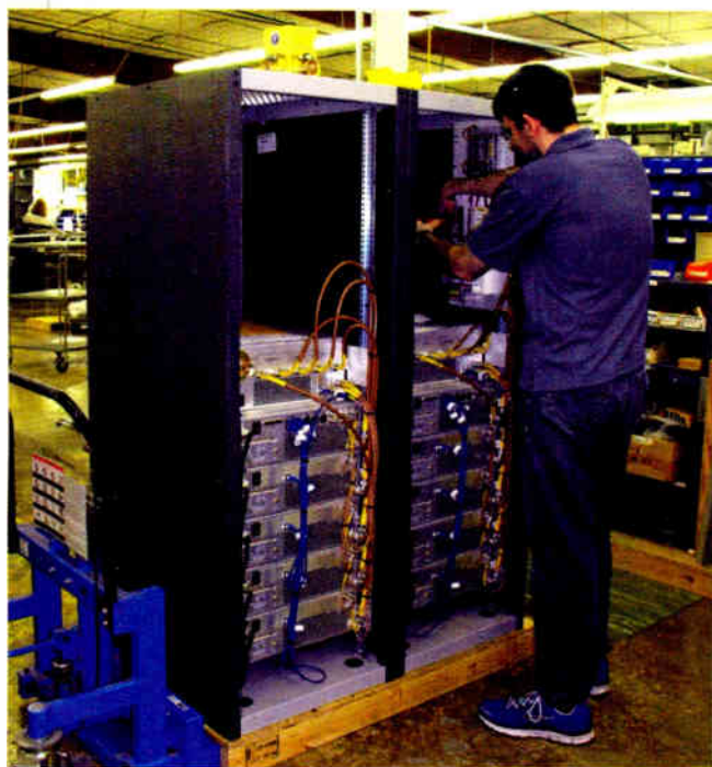
Jason Rouse, BE assembler, finishes the build of a 5 kW STX LP main/alternate radio transmitter system.
