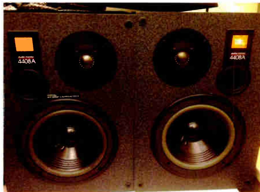
Fig. 5: The repaired woofer is on the left.
