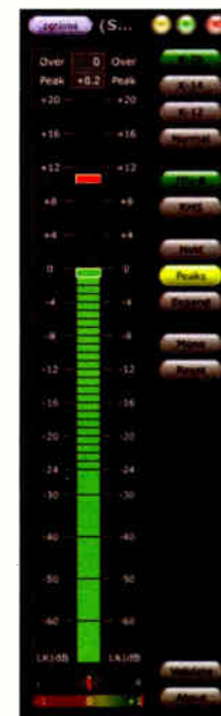
Fig. 3: In this screenshot of the K-Meter, a program for Windows and Unix computers, ITU loudness is indicated by the solid green bar while the momentary signal peak is shown by a single red segment.
