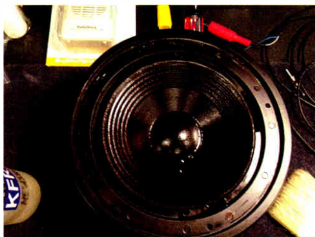
Fig. 3: Clean surfaces are ready for test fitting of the new foam surround.
