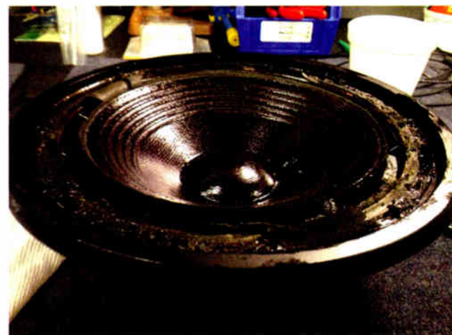
Fig. 2: Removing the old foam surround can be a little intimidating.
