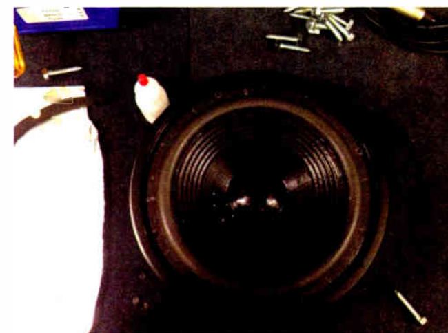
Fig. 4: Centering the speaker coil is important prior to gluing the outer edge of the surround.
