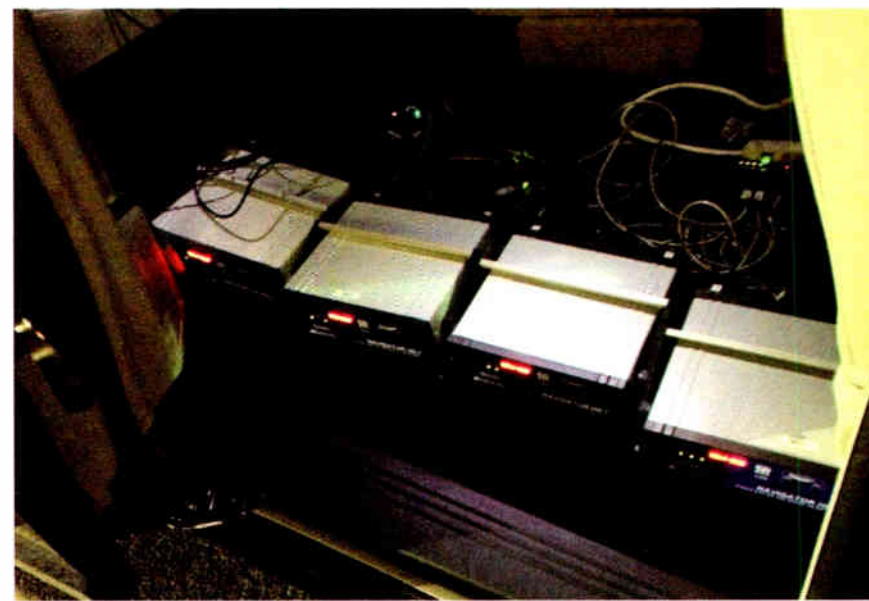
Rear of the vehicle showing the four Audemat Navigator HD units used for data coverage logging.
