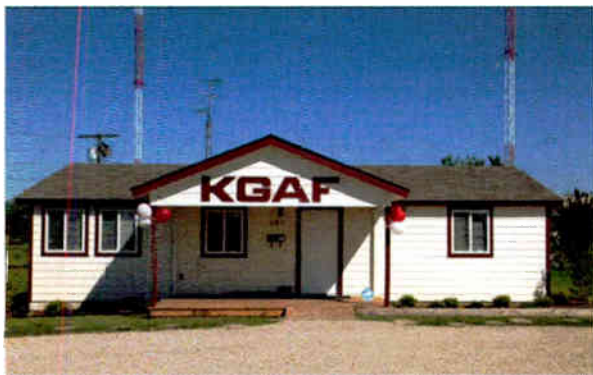
This shows the current KGAF building, which was constructed in 2009, replacing the original 1947 building. It shows the two towers, 200 ft. tall, each located on the same property. The station is 250 watts non-directional daytime; 250 watts directional two-tower array at night.
