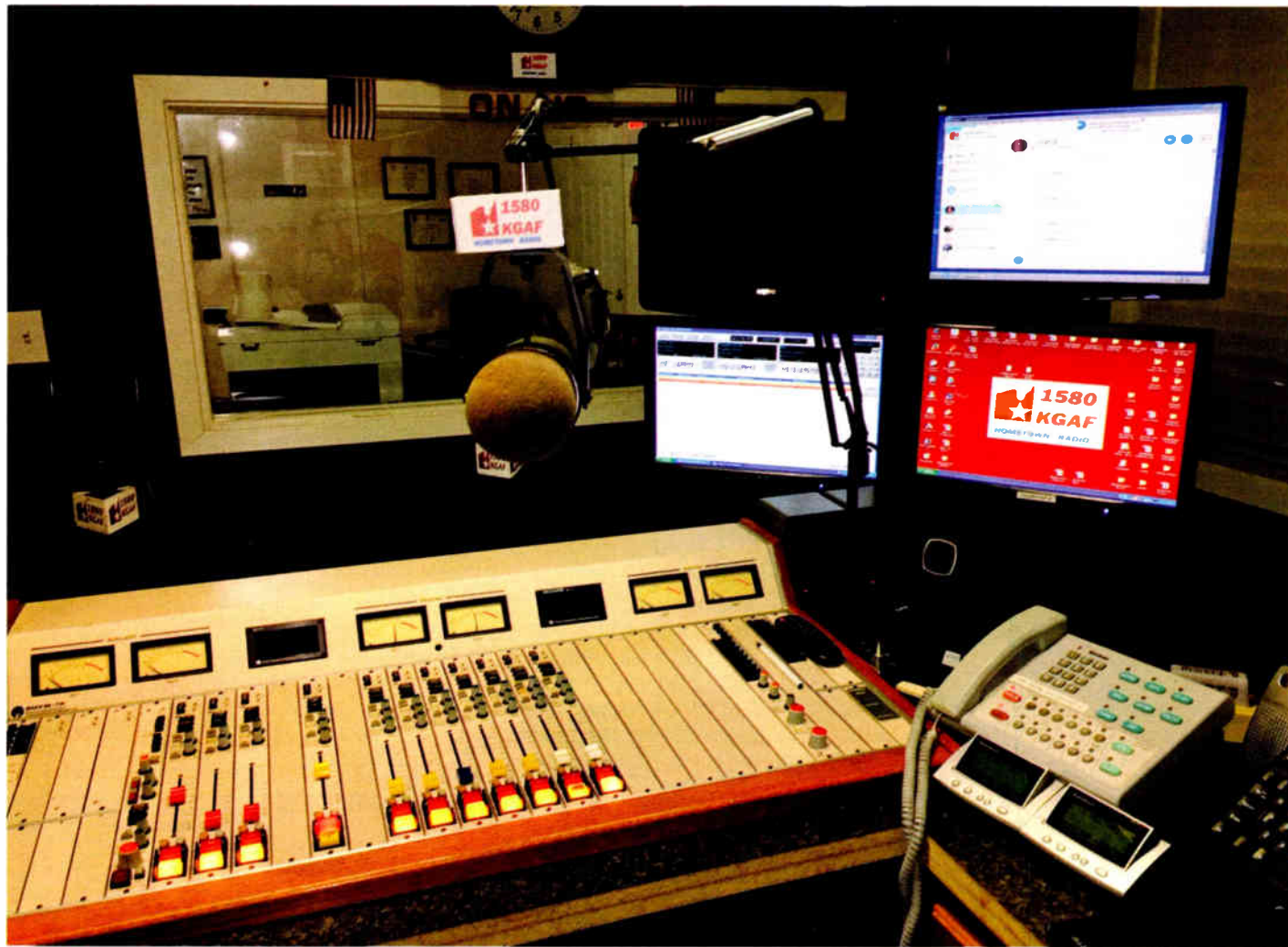
The Pacific Recorders BMXIII console, 11 Software Jockey Pro automation on the computer screen, three Shure SM 5-B microphones, Gentner TS-612 broadcast phone system and Fostex powered monitors. Eberhart also notes that this picture shows the "only real relic from the original 1947 building, the "ON AIR" light, which we restored and works!"
