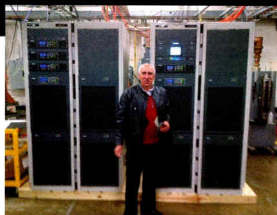
Nova FM Director of Technology Teodoro Fonseca in front of the Flexiva 80 kW transmitter during the testing phase at GatesAir's manufacturing center.
